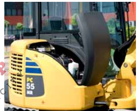
Front bonnet: fuel tank refilling
