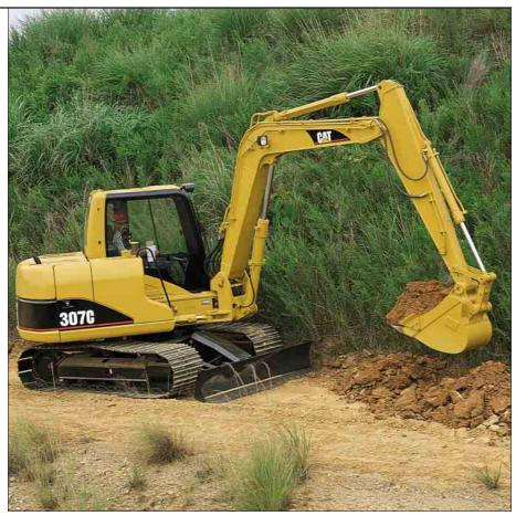
**Buckets.** High tensile strength steel is used in high-stress areas for excellent wear and shock resistance. The side plates are tapered to prevent contact of the bucket sidewalls during trenching operations.
